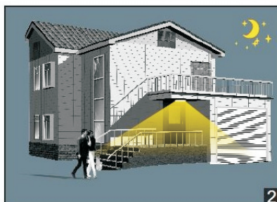
2 With insufficient daylight,even when motion detected.light ON.
